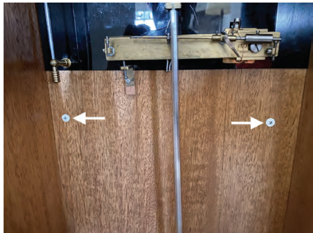
Figure 1-5 Screws holding the case to the wall
