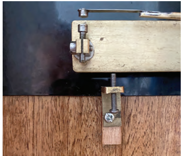
Figure 7-9 The new toggle stop
