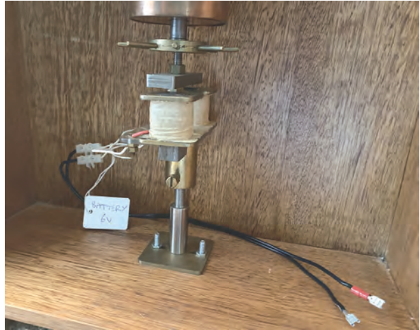
Figure 4-4 Electromagnet after wiring tidied up
