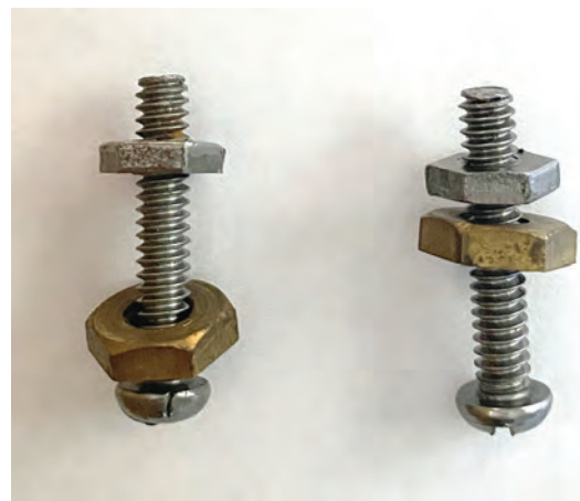
Figure 4-6 Old bolts holding the electromagnet
