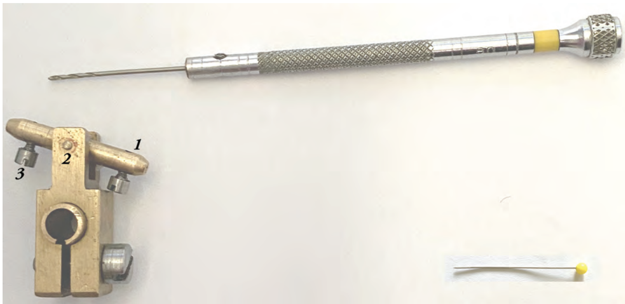
Figure 6-4 - Drilling for a new wire lever D
