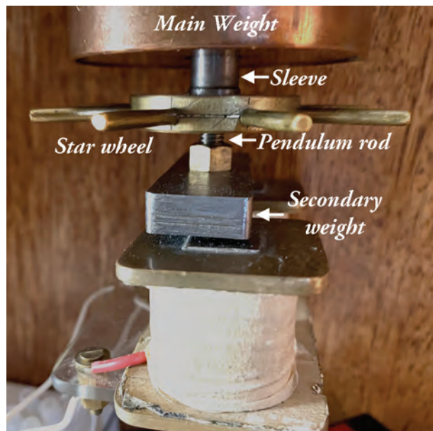
Figure 5-6 Action of the Star Wheel
