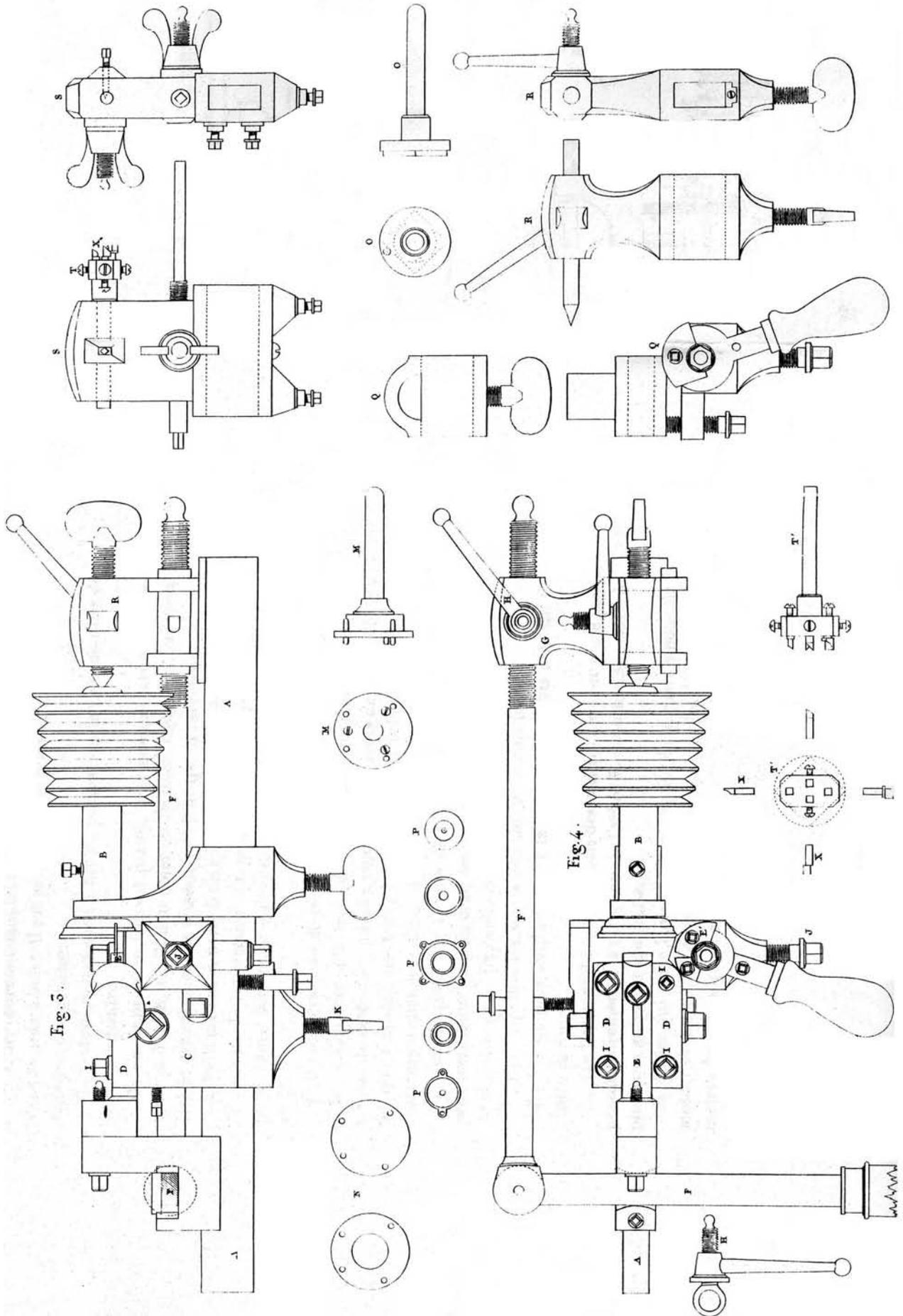
**Figures 5, 6 and 7:** Elevation and plan of a machine to cut the teeth of watch wheels.
